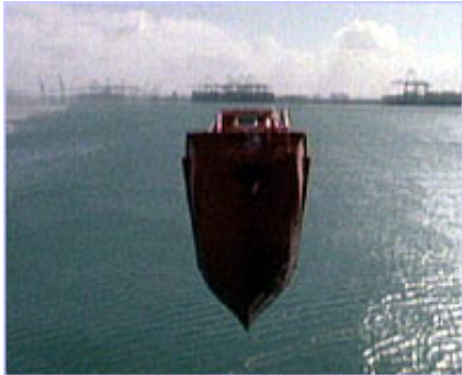
Verhoef's free fall lifeboat swiftly slides from its lodging on an oil platform...
