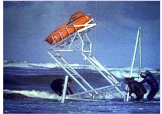
Early tests on this life boat demonstrated that it was self-righting and reliable.
